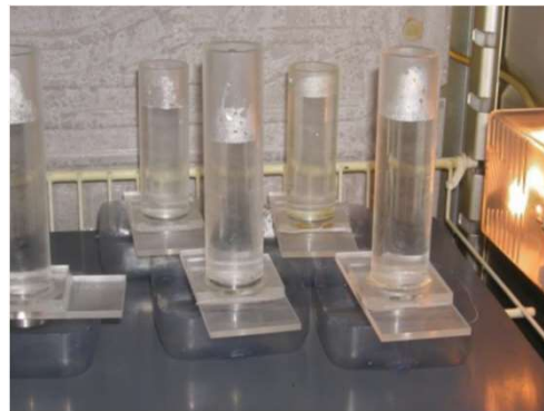
Sedimentation of fixed samples (Utermöhl method)
